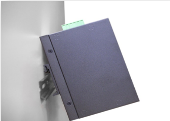
Figure 3.2 - Insert the Switch on the DIN-Rail
